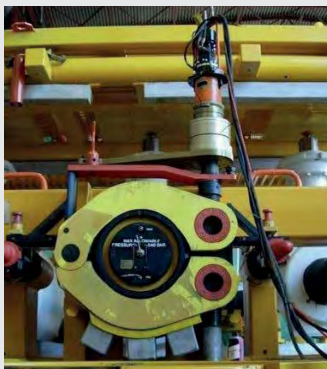
Wet Pipe Clamp Tool under test
